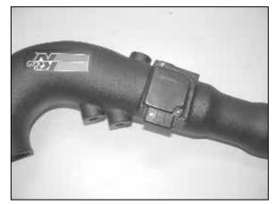
17. Secure the mass air sensor to the K&N<sup>®</sup> intake tube using the provided screws and spacers as shown.
