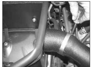
20. Secure the K&N<sup>®</sup> intake tube to the saddle
