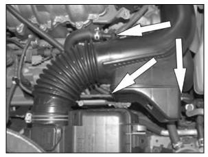
4. Remove the three vent lines from the air intake resonator as shown.
