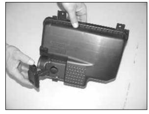
15. Remove the two screws that secure the mass air sensor to the air box lid, then remove the mass air sensor as shown.
