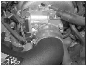
19. Install the K&N<sup>®</sup> intake tube onto the throttle body and align with the saddle bracket.
