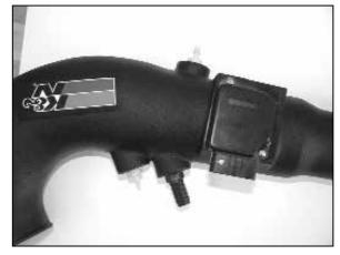
18. Assemble the vent fittings onto the  $K\&N^{\circledast}$  intake tube as shown.
