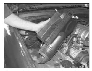
7. Remove the three bolts that retain the air box to vehicle, then remove the air box. NOTE: K&N Engineering, Inc., recommends that customers do not discard factory air intake.
