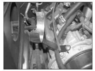
13. Install the saddle bracket assembly onto the threaded boss on the cam cover with the provided hardware as shown.
