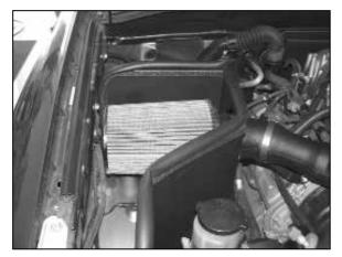
22. Install the K&N $^{\ensuremath{\mathbb{R}}}$  air filter onto the intake tube as shown.
