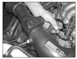
21. Install the provided silicone hose onto the K&N<sup>®</sup> intake tube and re-connect the one existing vent line as shown.
