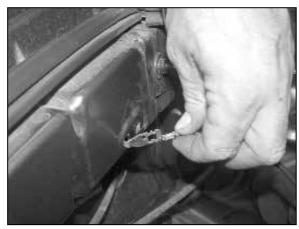
23. Disconnect the ground strap that's attached to the mass air sensor wiring harness at the inner fender as shown.
